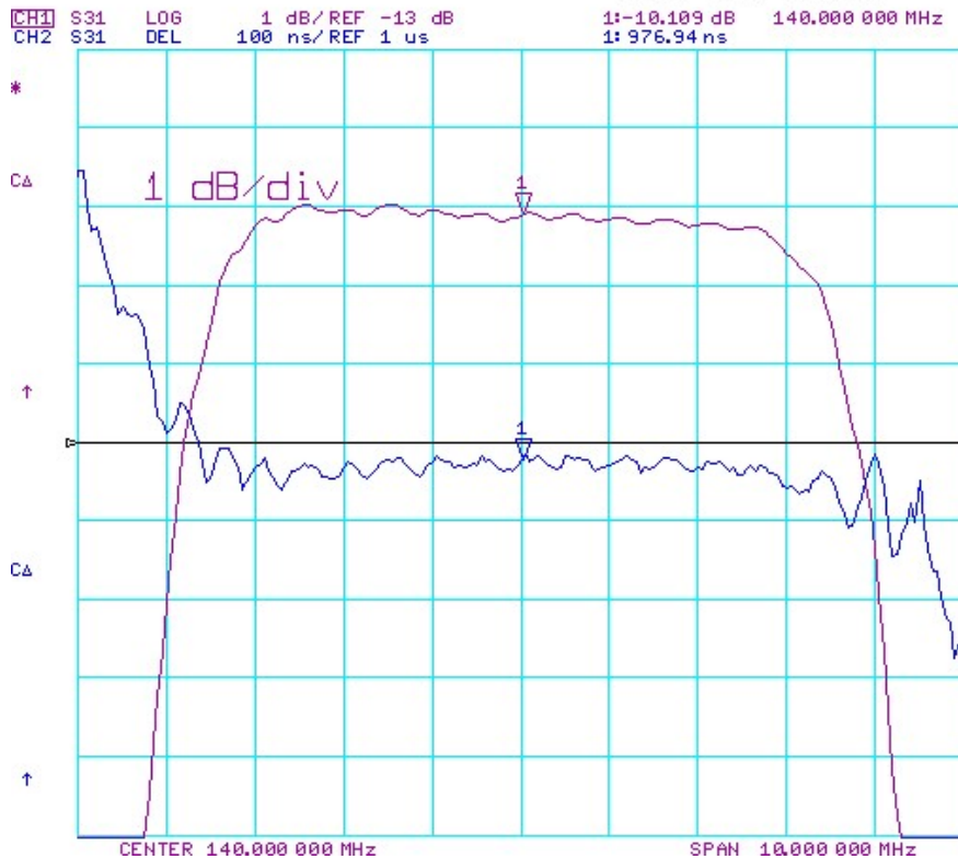
Fig2.S21 Response Horizontal:1MHz/Div Vertical: 1dB/Div
